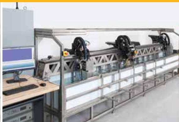
The latest in immersion ultrasonic testing assures defect free materials are used prior to machining.
